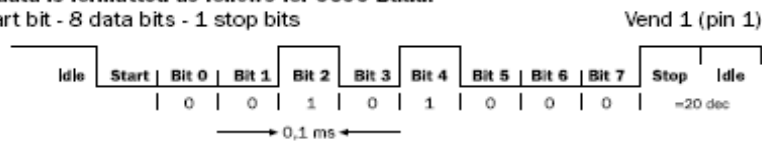
Figure 9 - Typical Serial Output: Transmission of the value 20 (decimal), note not recognized
